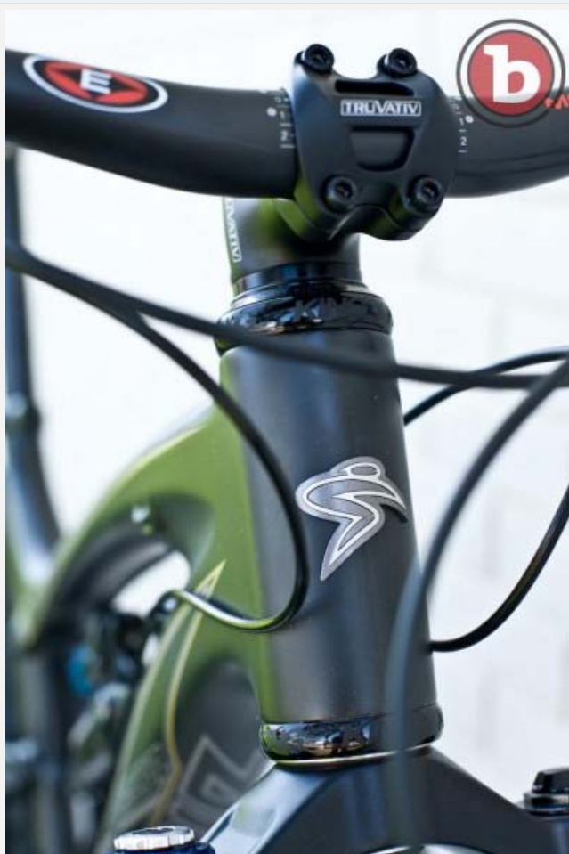
The Nomad Carbon receives a 1.5-inch headtube for improved stiffness and compatibility with any steerer configuration.
