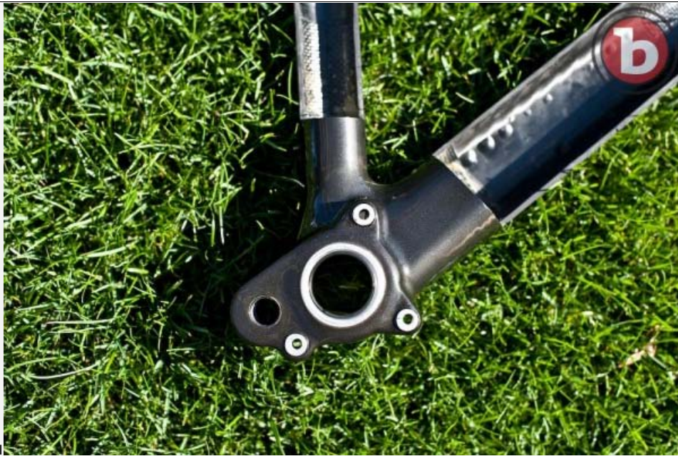
ISCG05 tabs are molded in the true one-piece carbon mainframe.
